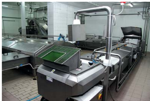
BATH & BRINING LINE - RASSODAMENTO E SALAMOIA Mod. ML/MS
