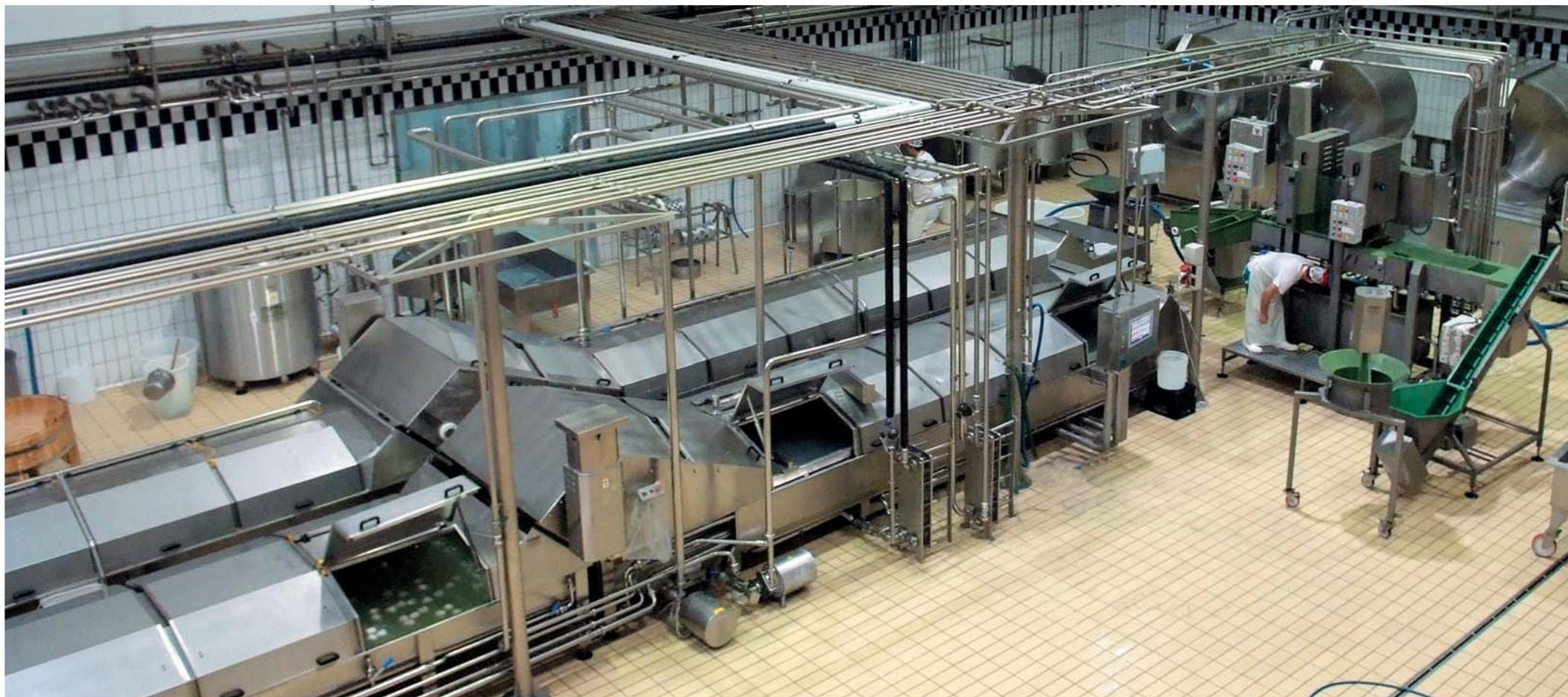
BATH & BRINING LINE - RASSODAMENTO E SALAMOIA Mod. ML/MS
